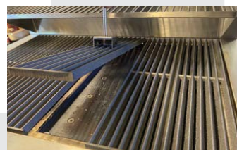
Using the lifter replace the bars
