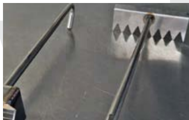
Scraping tool: Removes carbon build up Lifter: Lifts the bars off the grill safely
