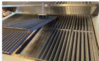
Using the lifter replace the bars
