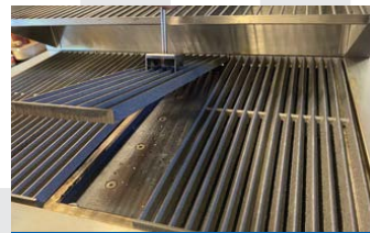
Using the lifter replace the bars
