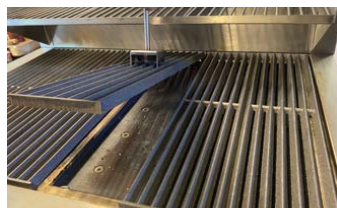
Using the lifter replace the bars
