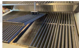
Using the lifter replace the bars
